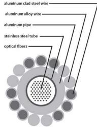
Figure 1: OPGW Cross-Section
