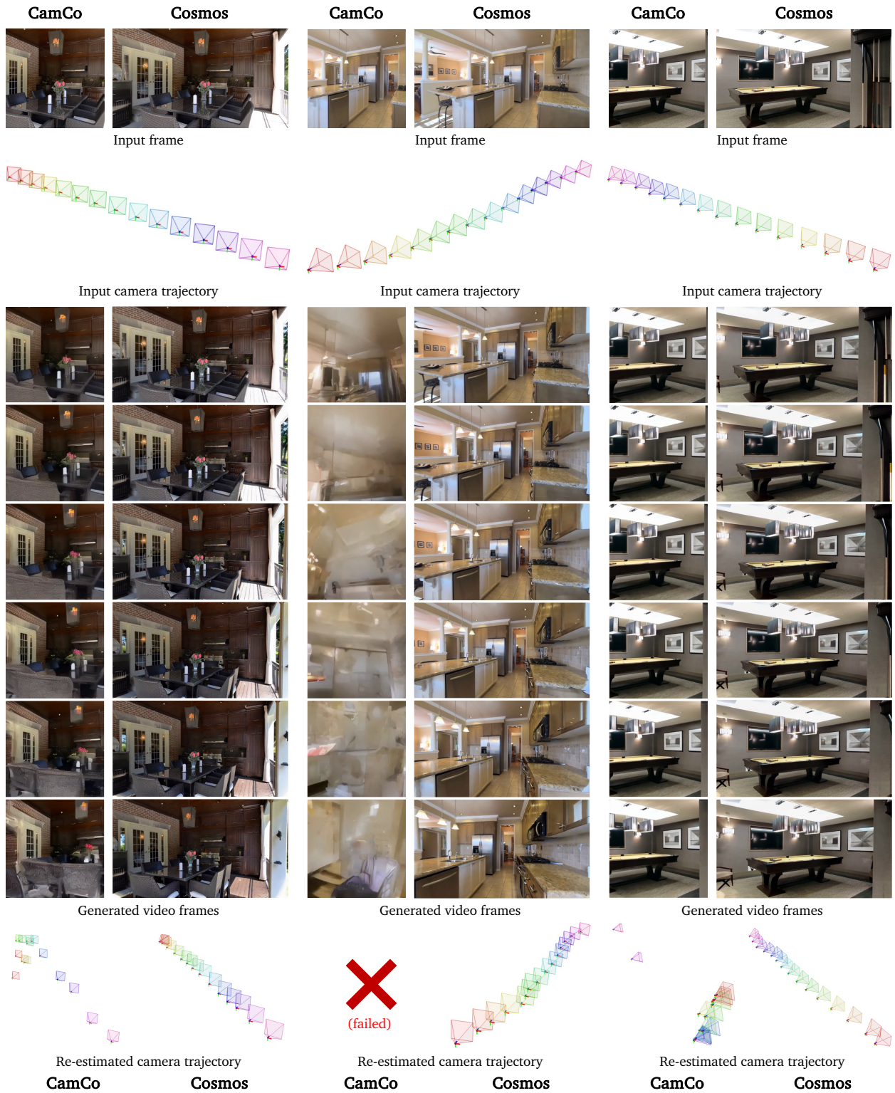
Figure 21: Qualitative comparison of camera control models. Given the input frame and camera trajectory (color-coded temporally from red to violet), we compare Cosmos-1.0-Diffusion-7B-Video2World-Sample-CameraCond against CamCo (Xu et al., 2024) on the generated future frames as well as the re-estimated camera poses. CamCo suffers from the data distribution shift and often generates inaccurate trajectories or even out-of-distribution image syntheses that lead to un-estimatable camera poses. In contrast, the Cosmos camera control model can successfully generate future frames aligned with the camera control input while also maintaining high video quality and 3D consistency.
