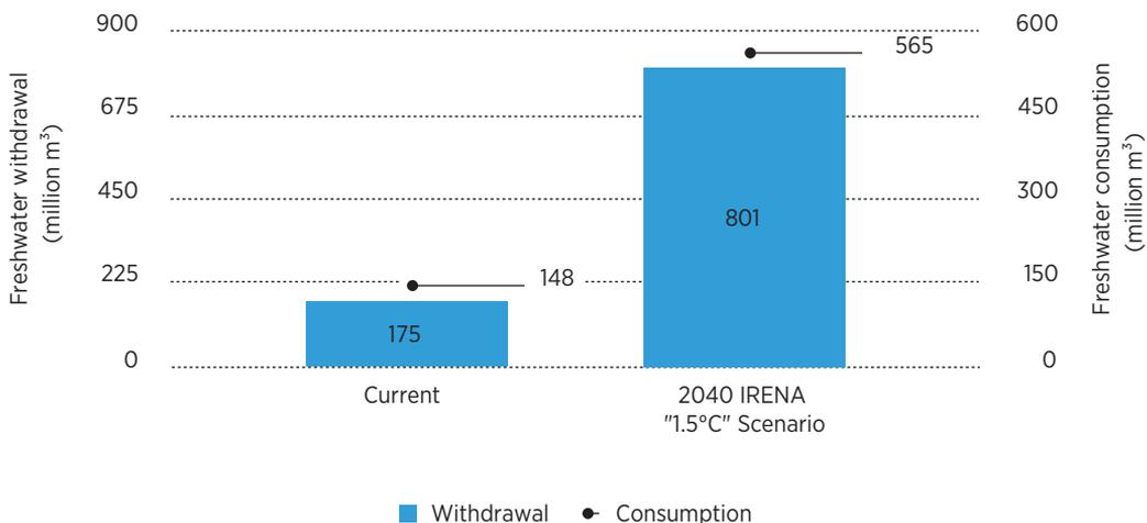
**Note:** Key assumptions include: (1) all cooling systems are freshwater evaporative systems; (2) for electrolysis, 50% alkaline and 50% PEM by 2040; (3) for natural gas with CCS, 50% SMR+CCS and 50% ATR+CCS by 2040; and (4) no seawater cooling or desalination for production water. ATR = autothermal reforming; CCS = carbon capture and storage; PEM = proton exchange membrane; SMR = steam methane reforming.
