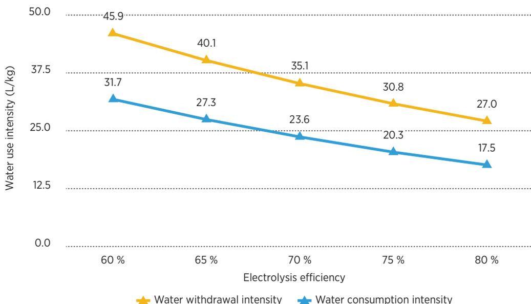
**Note:** The curves are estimated based on water balance modelling for a typical green hydrogen project with all system variables kept constant except efficiency. The system assumptions are the same as mentioned in the note of Figure 2.1. kg = kilogramme; L = litre.
